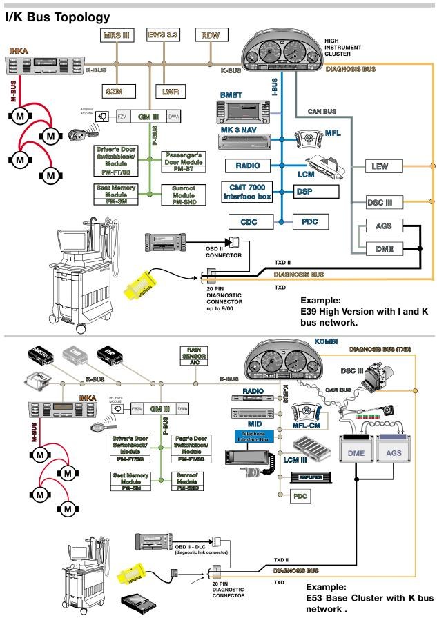
The I/K bus consists of a single copper wire. The wire color of the I and K bus is uniform throughout the vehicle with: I-bus WS/GR/GE and the K-bus WS/RT/GE (Note: 2001 E39s with base Kombi have changed K-bus wire color to the same as the I-bus, WS/GR/GE).
